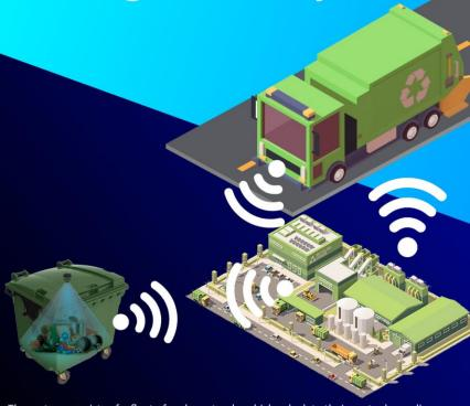
The system consists of a fleet of garbage trucks which calculate their route depending on how much garbage has accumulated in each container that is present throughout the city. Sensors are placed in the garbage containers; these sensors estimate how full containers are and they relay the information to a central operations base, where the decision to collect the garbage is made.
